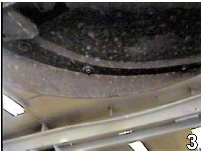
3. Using the 6MM socket, remove three metric bolts, just forward of the front tire. Set metric bolts aside to be reinstalled later. Do this to both sides of the vehicle.
